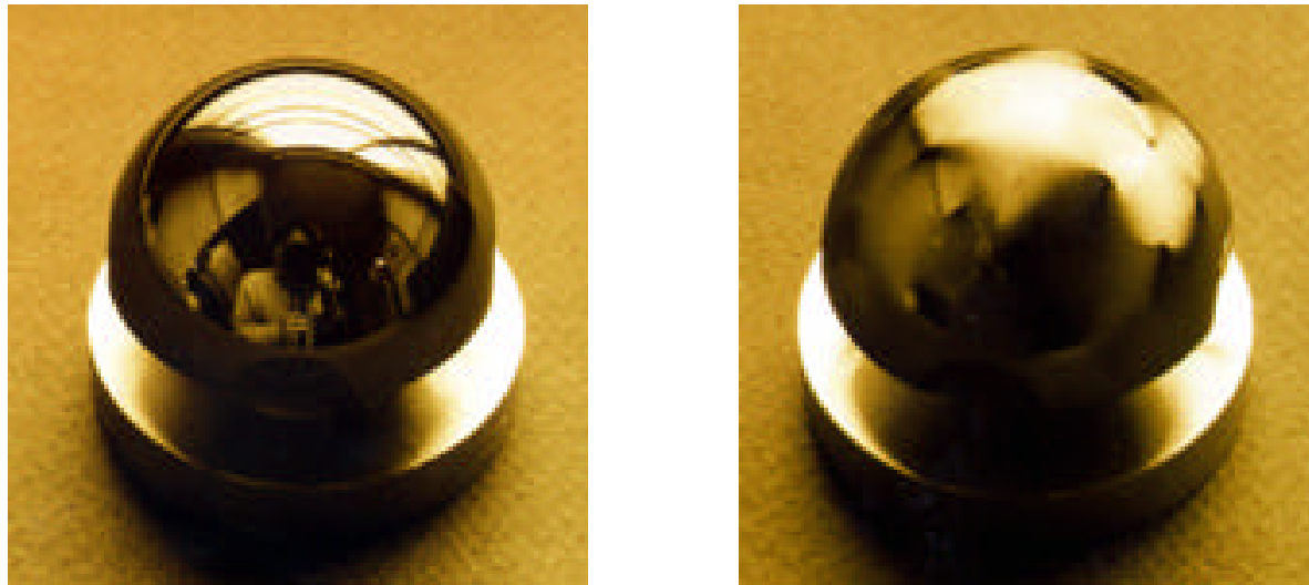
Fig.1 Silicon test piece before and after etching
